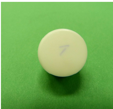
Sketch 3: prepared test specimen, sample 1 Abrasion surface for testing
